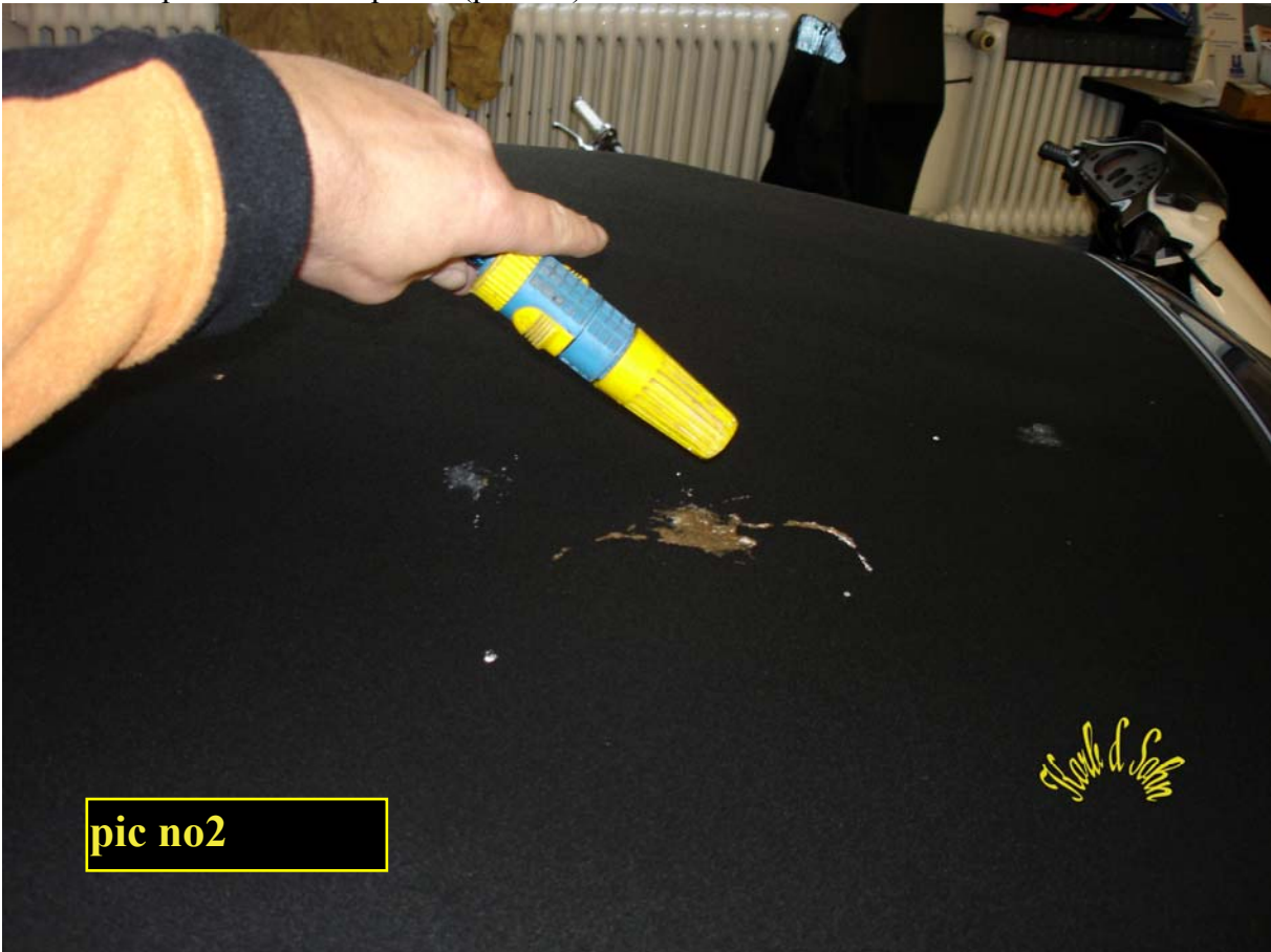
The first step is to soak the points (pic no2)
